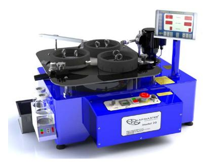
The Lapmaster Model 20 lapping / polishing machine is fitted with an electronic dispenser for the liquid diamond abrasive slurry and the appropriate lubricating fluid, a dual head spray bar and an electrically driven stirrer unit which houses small glass reservoirs of both fluids
